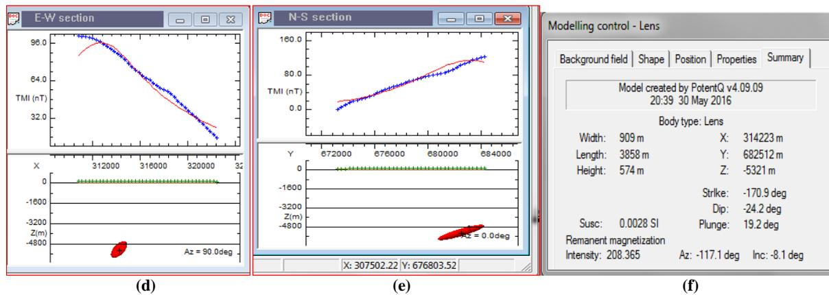
Fig 7(a – f): The complete results from profile 2(a) Observed plan(b) calculated plan (c) Residual Plan (d) Graph of E-W section (e) Graph of N-S section (f) Summary of the modeling
