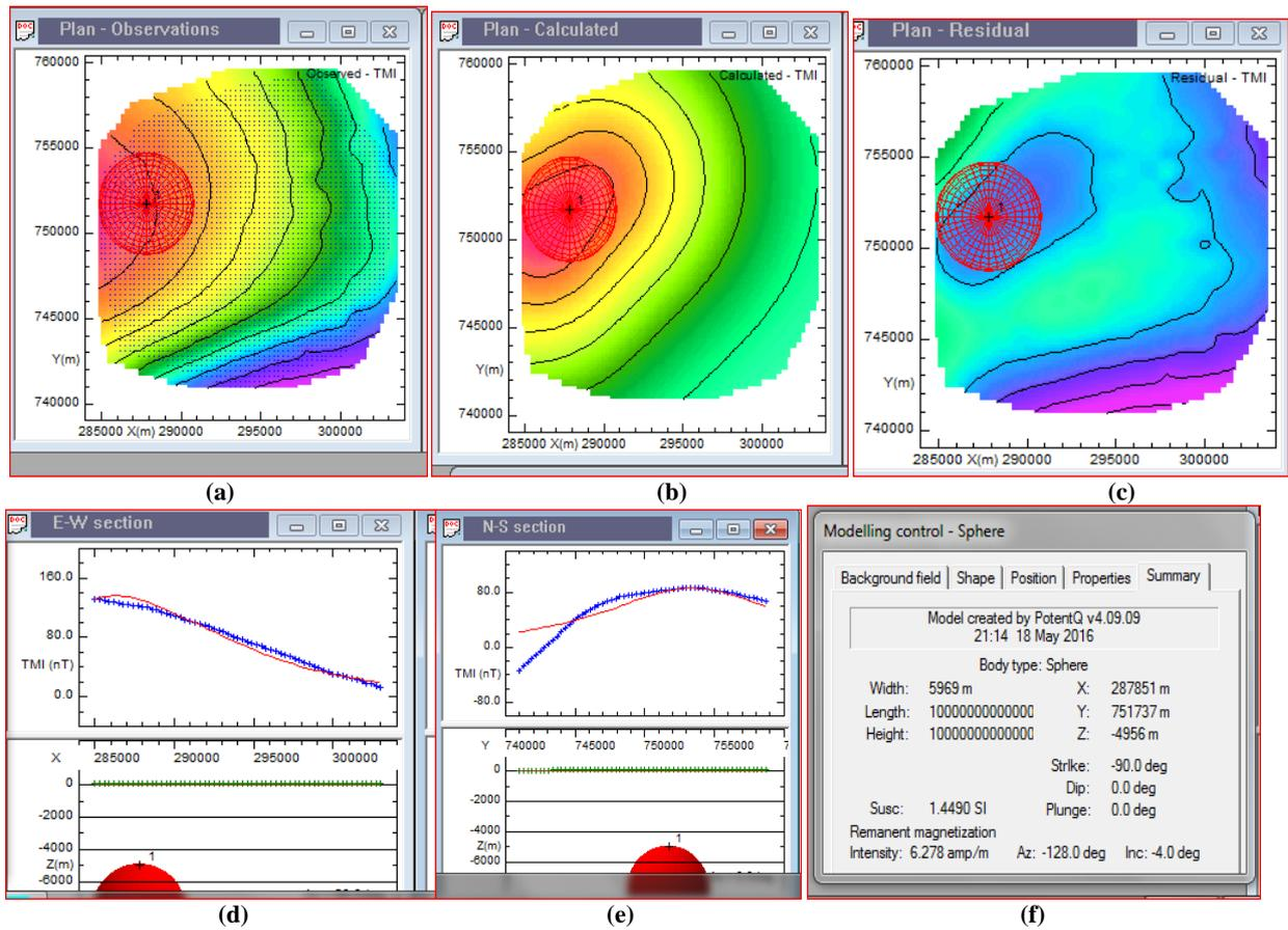
Fig. 6(a – f): The complete Results from Profile 1(a) Observed plan, (b) calculated plan, (c) Residual Plan, d. Graph of E-W section, (e) Graph of N-S section, (f) Summary of the modeling
