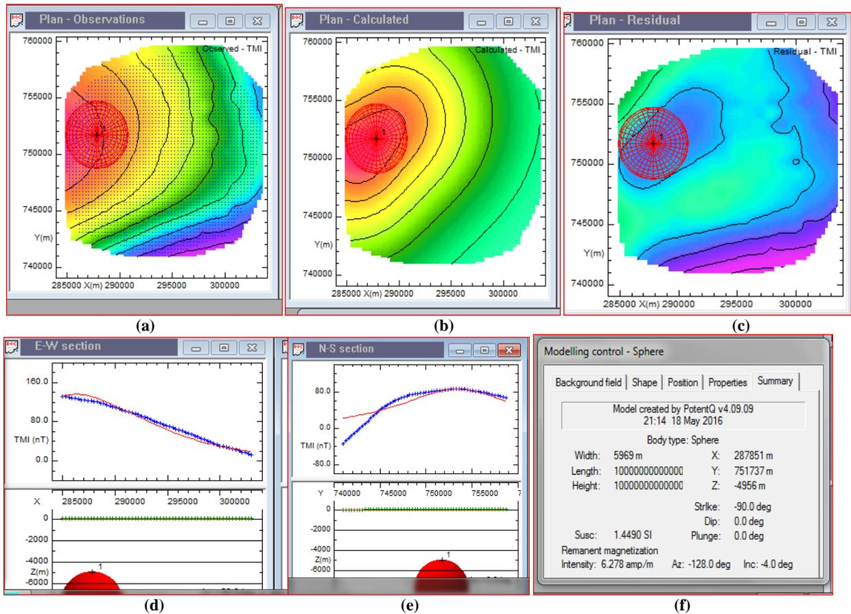
Fig. 6(a – f): The complete Results from Profile 1(a) Observed plan, (b) calculated plan, (c) Residual Plan, d. Graph of E-W section, (e) Graph of N-S section, (f) Summary of the modeling
