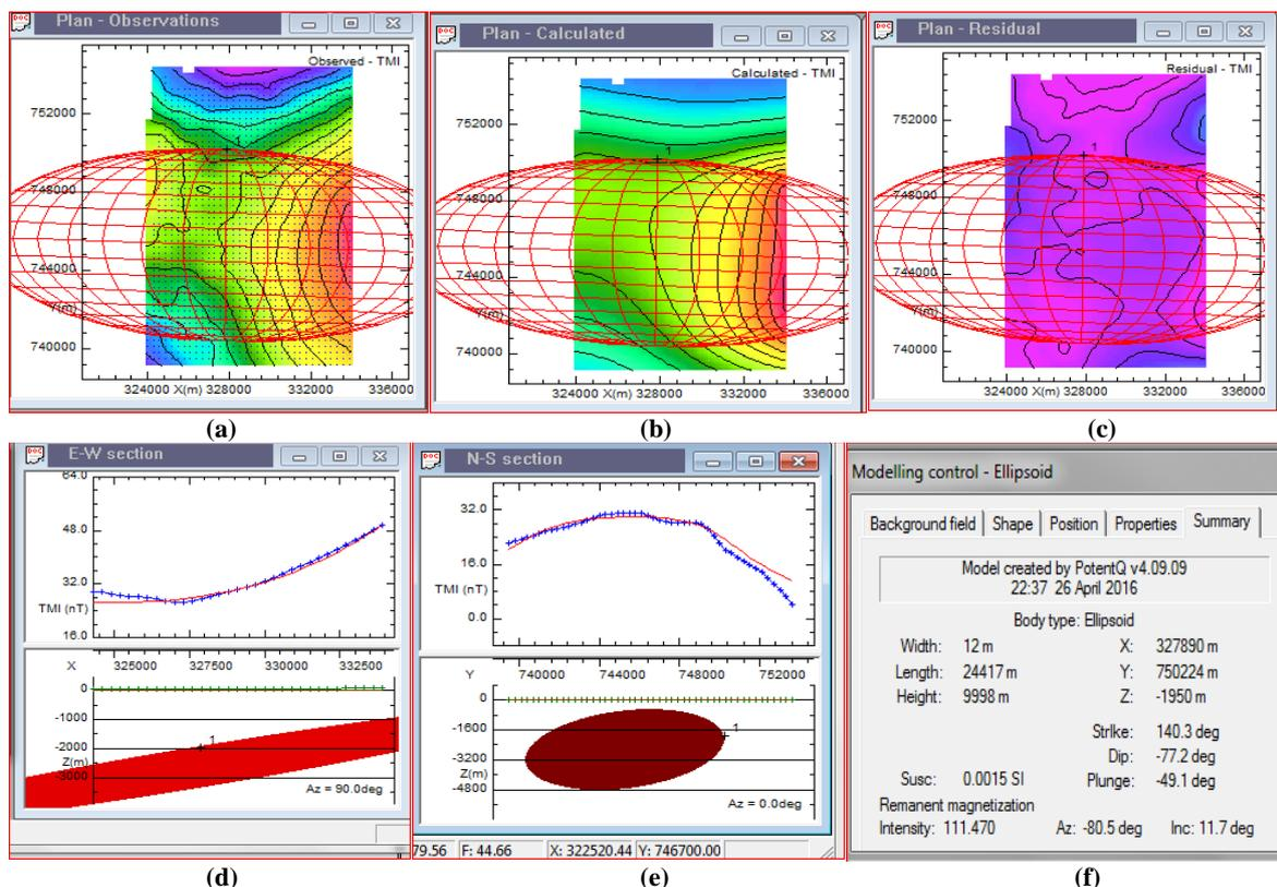
Fig 8(a – f): The complete results of profile 3(a) Observed plan (b) Calculated plan (c) Residual Plan (d) Graph of E-W section (e) Graph of N-S section (f) Summary of the modeling
